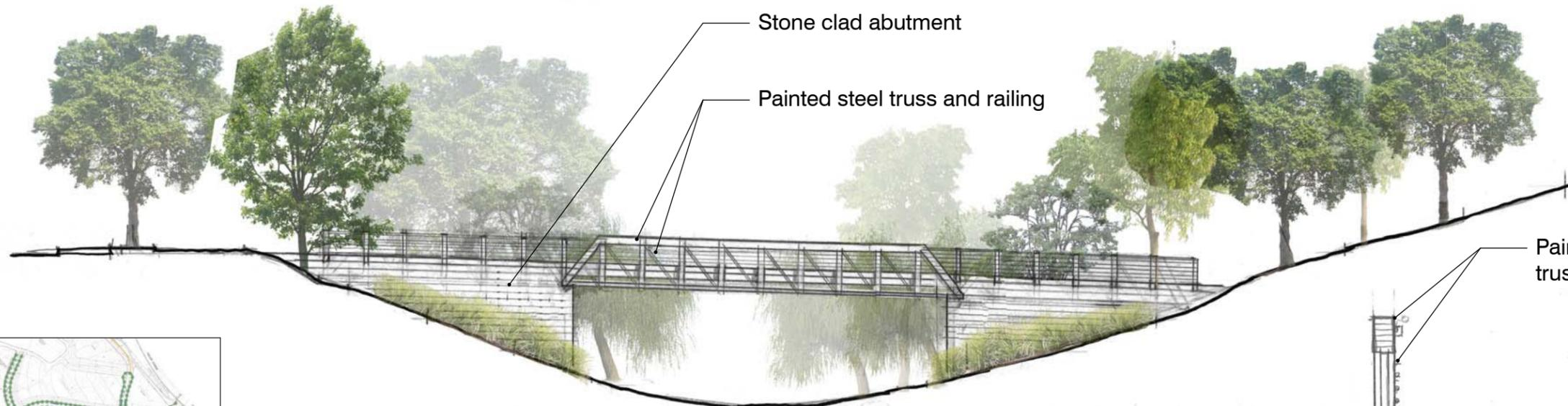
Painted steel truss and railing
