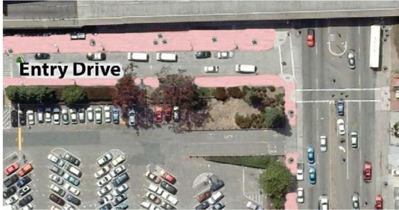
another lane to pass the stopped vehicles. That means that there are two vehicle lanes in one direction to allowing passing and stopping without interrupting traffic flow.
