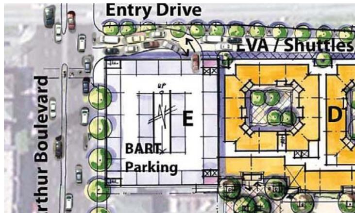
At this scale it is difficult to determine how the ped-bike multi-use path from MacArthur to the BART station on Entry Drive’s west side would work. It appears that the driveway, to enhance the entry to the parking garage, has intruded the pedestrian path. This needs to be corrected and a minimum 10-foot wide (12-foot preferred) multi-use path should be built to convey pedestrians and bicyclists to and from the station. Pedestrian friendly surfacing should be provided.
