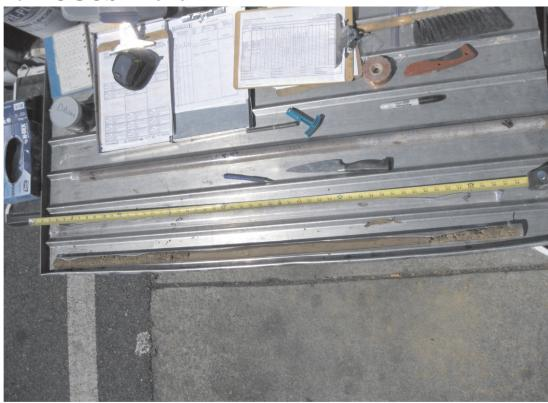
Photograph 14: Soil Sample, Boring B-02, 12 feet to 14 feet below ground surface.
