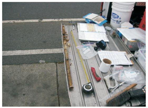
Photograph 2: Soil Sample, Boring B-01, 4 feet to 8 feet below ground surface.
