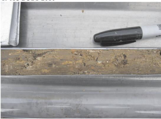
Photograph 5: Close-up of Soil from Boring B-01 at 11 feet below ground surface.
