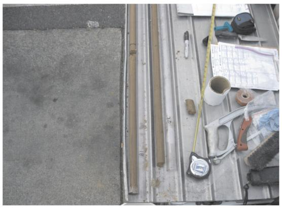
Photograph 6: Soil Sample, Boring B-01, 16 feet to 18 feet and 18 feet to 20 feet below ground surface.
