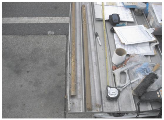
Photograph 4: Soil Sample, Boring B-01, 12 feet to 14 feet and 14 feet to 16 feet below ground surface.
