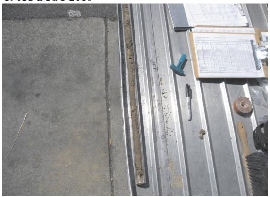
Photograph 12: Soil Sample, Boring B-02, 8 feet to 10 feet below ground surface.
