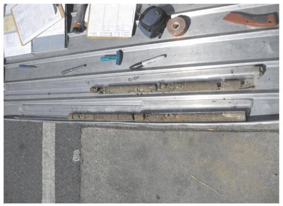
Photograph 11: Soil Sample, Boring B-02, 4 feet to 6 feet and 6 feet to 8 feet below ground surface.
