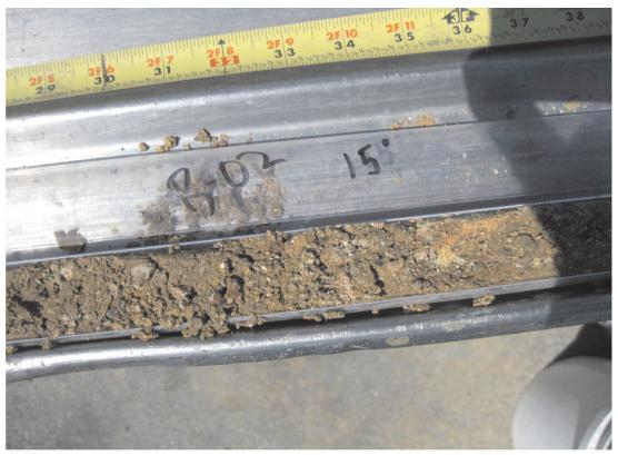
Photograph 17: Close up of Soil from Boring B-02 at 15 feet below ground surface.
