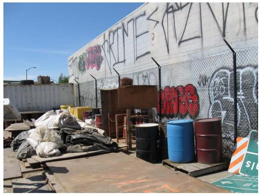
**Photograph 7:** Several drums potentially containing waste oil or coolant were present on the northeast corner of the Site (note lack of secondary containment).
