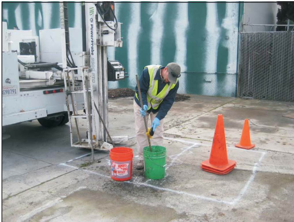
Photograph 10: TEG decontamination of probes removed from SG-04.
