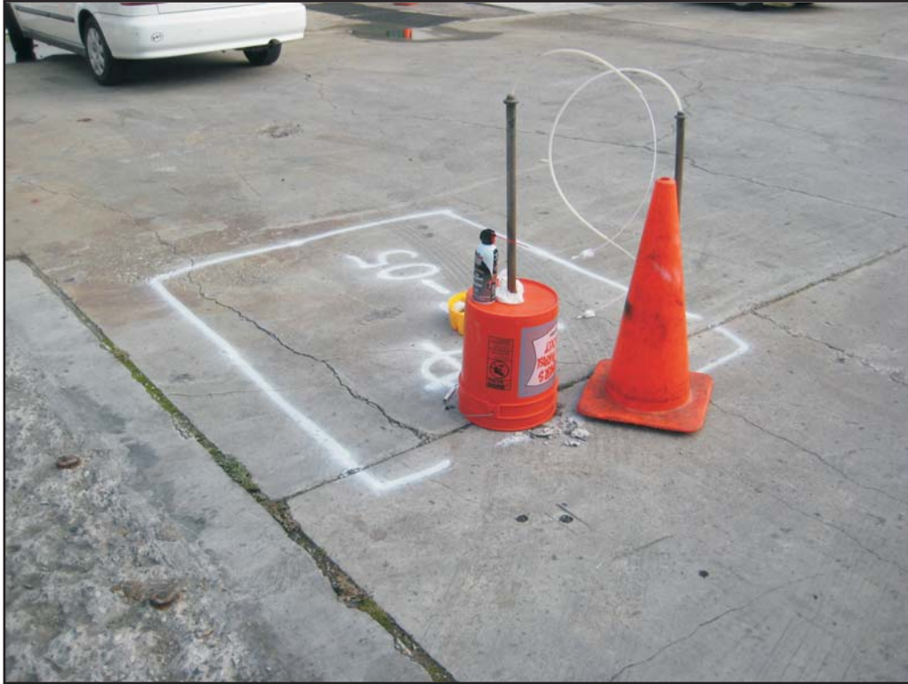
Photograph 11: Leak test at shallow probe at SG-05.
