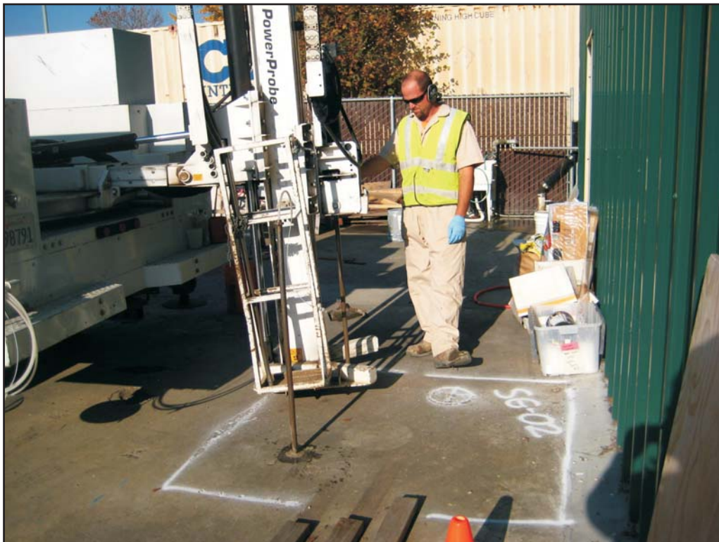
Photograph 28: TEG installing deep probe at SG-02.
