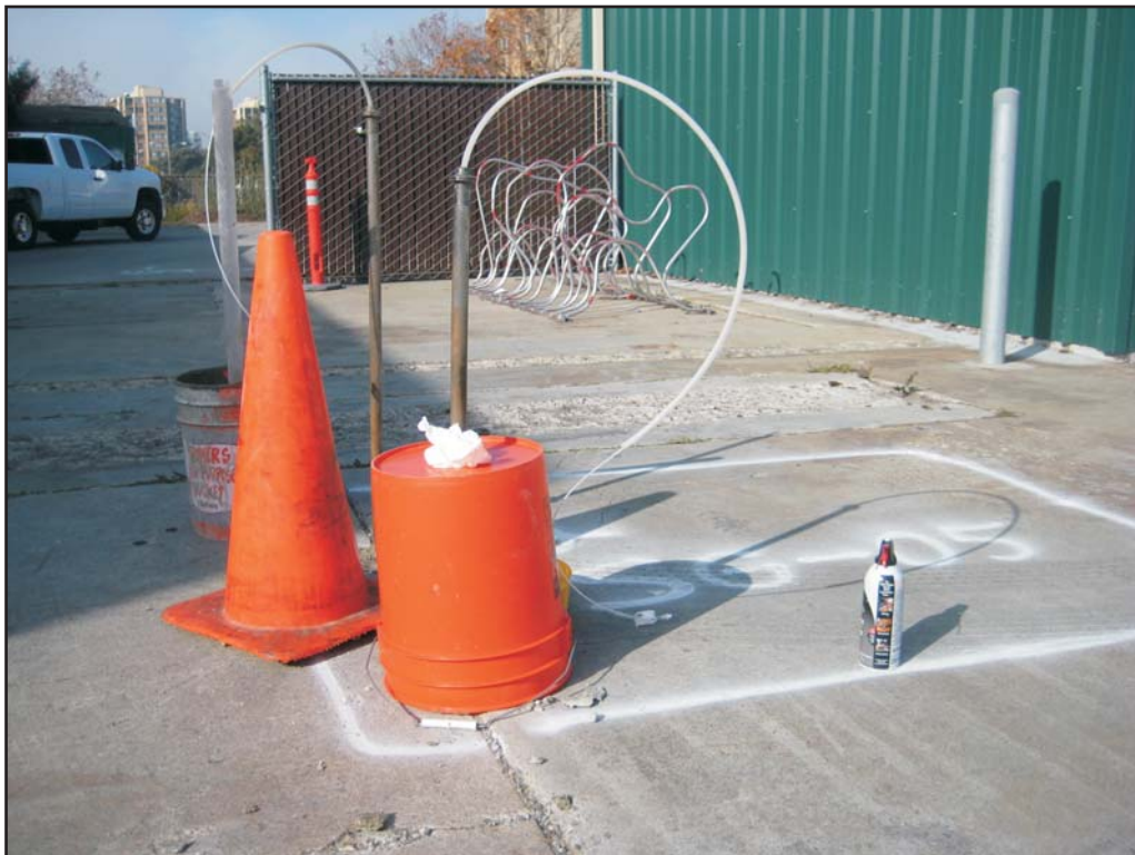
Photograph 14: Leak test at deep probe at SG-05.
