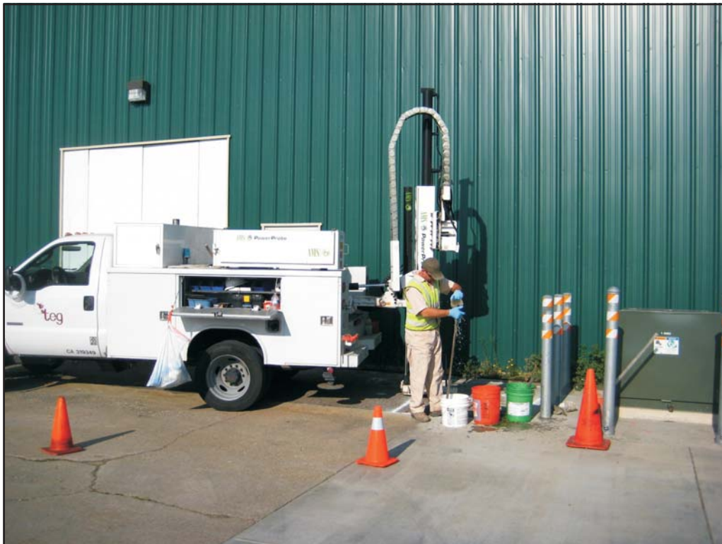
Photograph 24: TEG removing decontamination of probes from SG-01.
