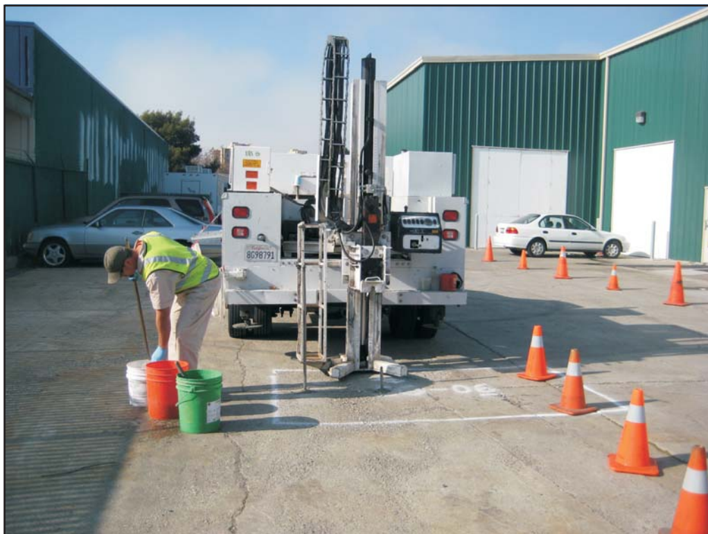
Photograph 20: TEG decontamination of probes at SG-06.
