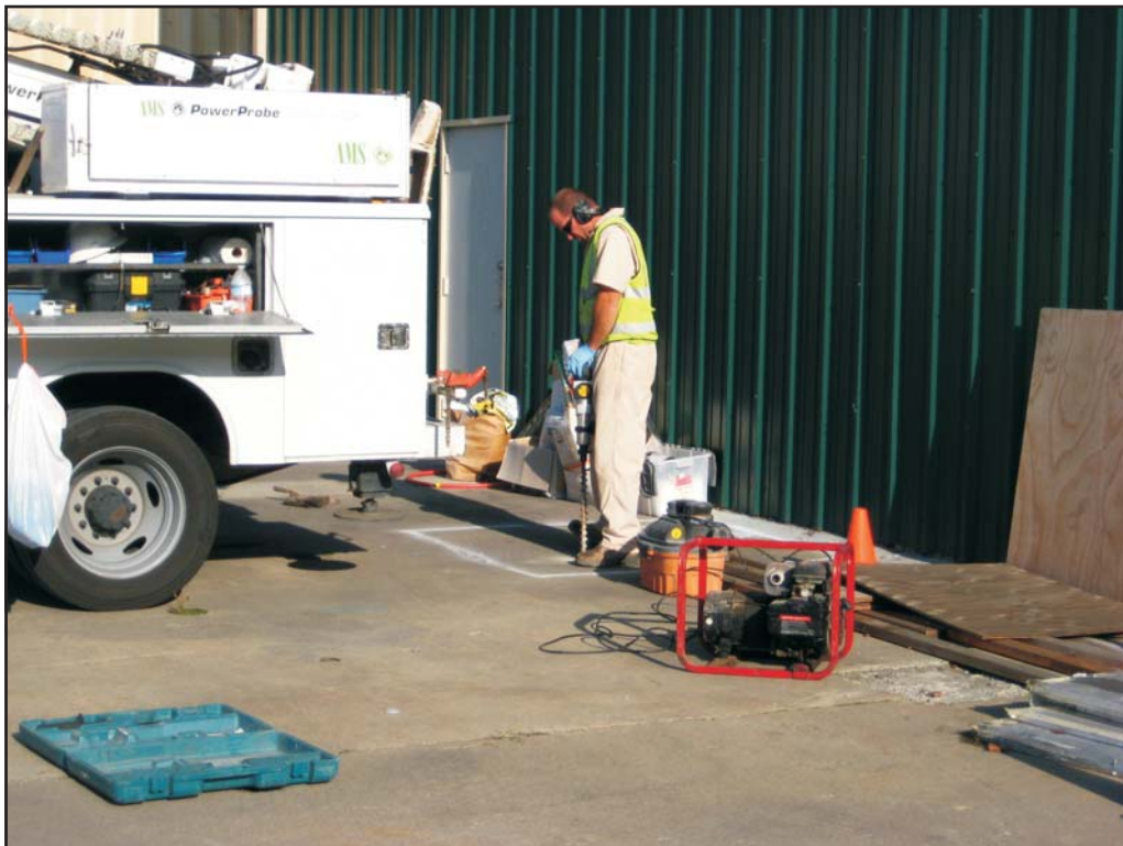
Photograph 26: TEG coring through pavement at SG-02.
