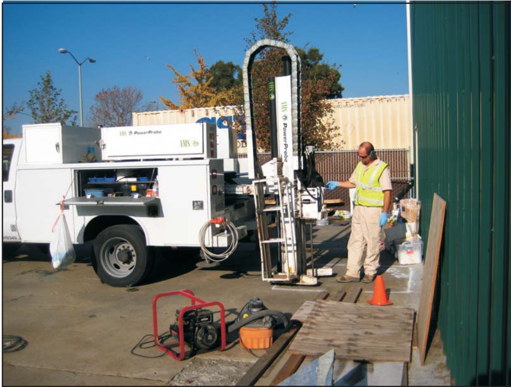
Photograph 27: TEG installing shallow probe at SG-02.
