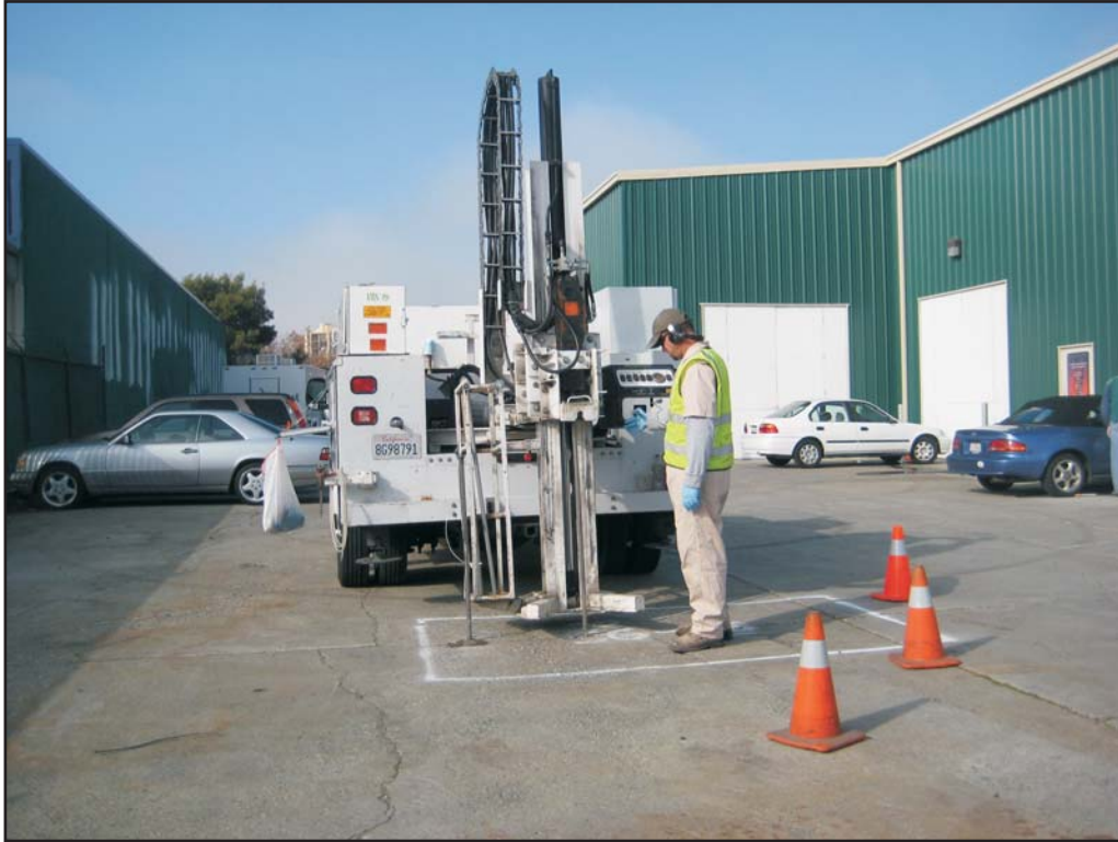
Photograph 13: TEG installing deep probe at SG-06.
