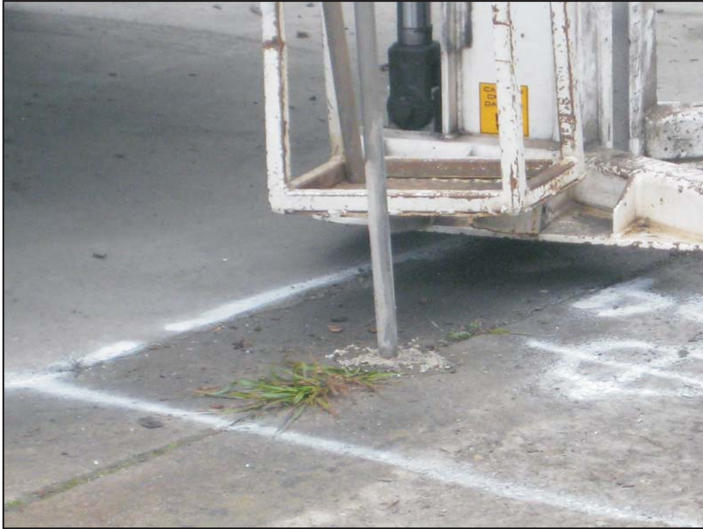
Photograph 5: Bentonite seal at ground surface at SG-04.
