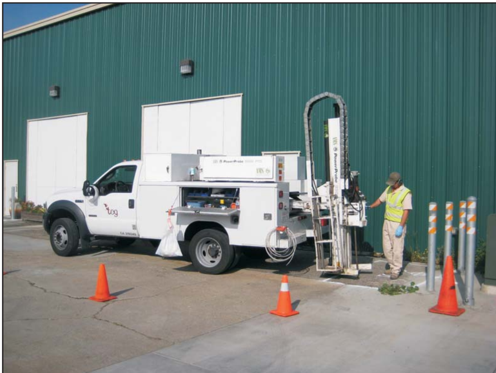
Photograph 18: TEG advancing shallow probe at SG-01.
