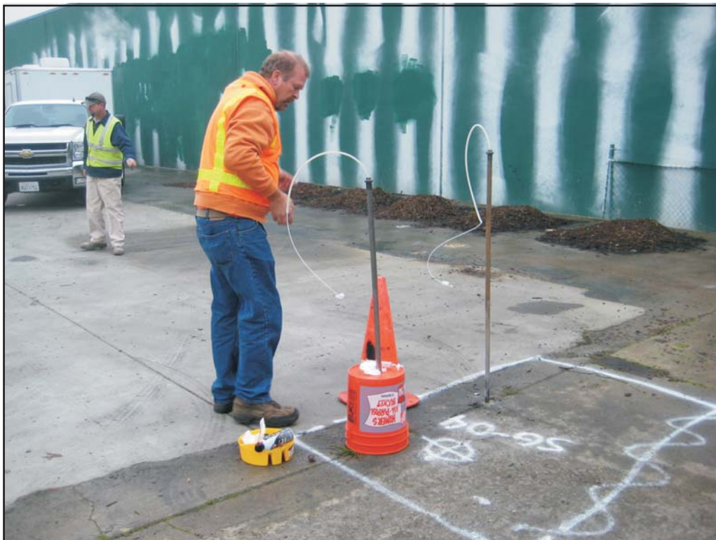
Photograph 6: TEG setting up for leak test at the shallow probe at SG-04.
