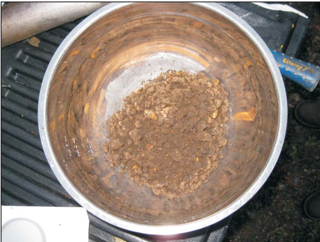
Photograph 4: Homogenization of sample from PH-10 using stainless steel bowl.
