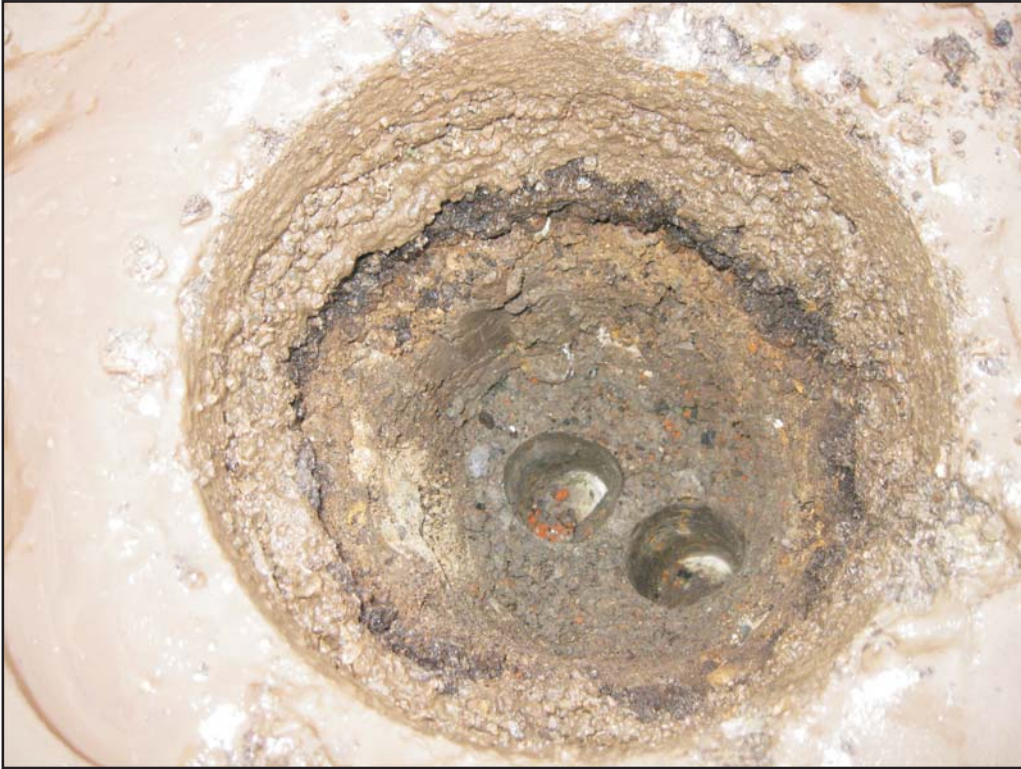
Photograph 1: Refusal at PH-01 at 15 inches below ground surface.
