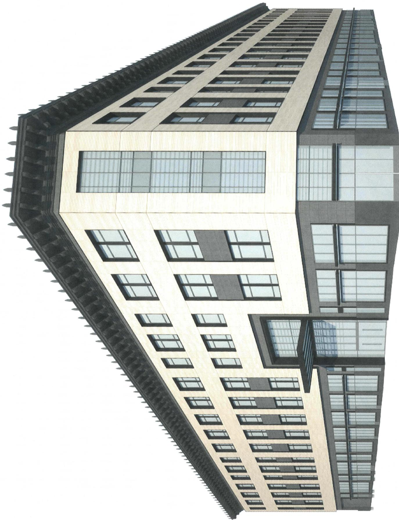
**CORNER SCHEME 8 - WRAPPED TERRA COTTA, NO REVEAL AT CORNERS WITH CURTAIN WALL**
