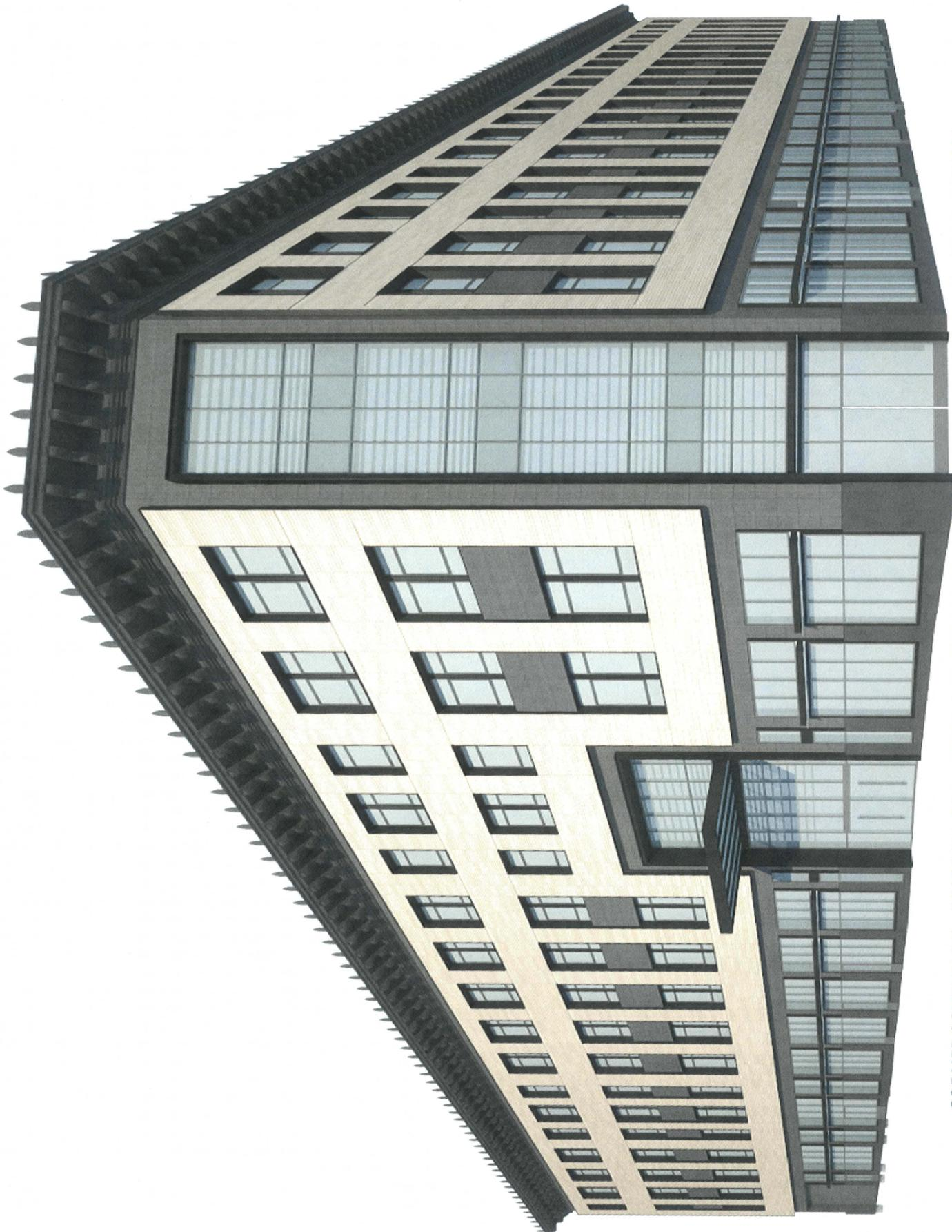
**CORNER SCHEME 6.2 - ORIGINAL CORNER SCHEME WITH EDGES OF TERRA COTTA PULLED BACK - CURTAIN WALL**
