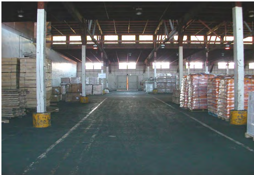
Figure 4.24. Building 808, transverse view of interior. Natural lighting is provided by the monitor windows and the lower window row over the loading bays. Note how the bay is on axis with the aisle formed by the rows of columns.
