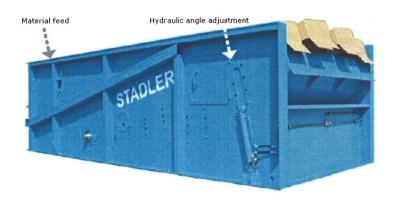
Separating of the most different material compositions in three material fractions. By throwing the material up and forward by a paddle, the Ballistic Separator sorts the materials due to their ballistic properties. A 90% precise material separation into heavy, screen and light fraction is achieved. In addition, the material is cleaned from dirt and dust.
