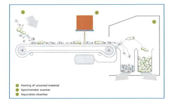
Input material (1) is evenly fed onto a conveyor belt, where it is detected by the NIR and/or VIS spectrometer based detector (2). If the sensors detect material to be sorted out, it commands the control unit to blow the appropriate valves of the ejection module at the end of the conveyor belt. The detected materials are separated from the material flow by jets of compressed air. The sorted material is divided into two or three fractions in the separation chamber (3).
